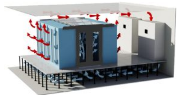
Cold Aisle Containment System with door at the front and the end of the row
